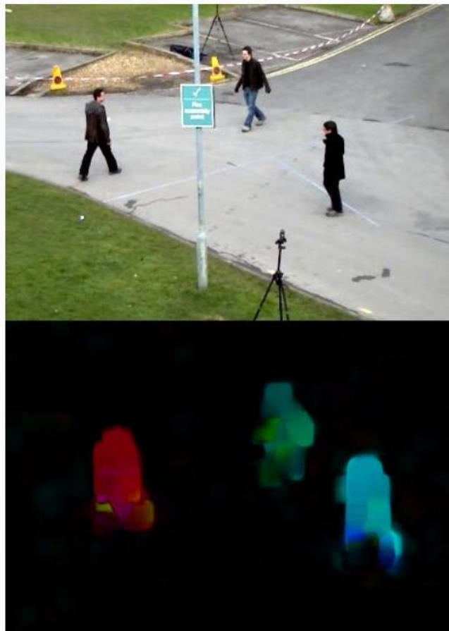
Figure 59: Dense Optical Flow (OpenCV, 2020)
