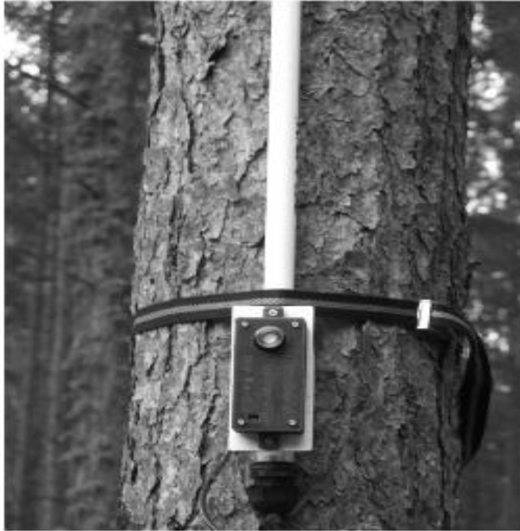
Figure 19: Hydrogen sensor mounted to a tree during an experiment done in Humboldt University in Berlin, Germany. (Nörthemann, Bienge, Müller, & Moritz, 2013)
